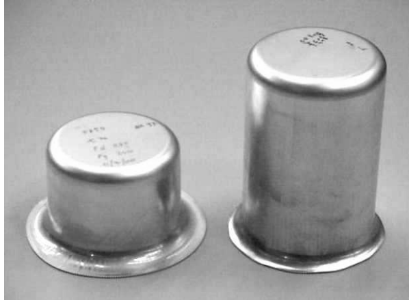
Figure 1.1: Maximum cup heights achieved at 20 °C (left) and with the flange at 250 °C (right) (courtesy TNO Industrial Technology).
